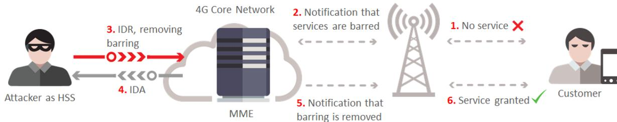
Figure 7 - Example of Fraud via S6a IDR
