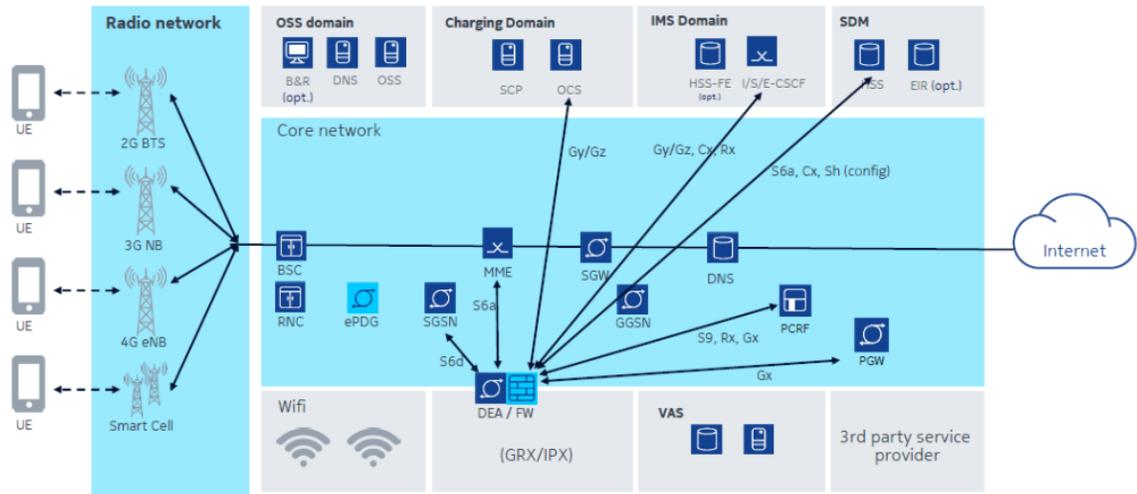
Figure 1 – Diameter Interfaces
