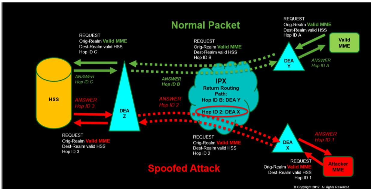
Figure 4 - Spoofing Vulnerability through Hop-to-Hop Authentication<sup>10</sup>
