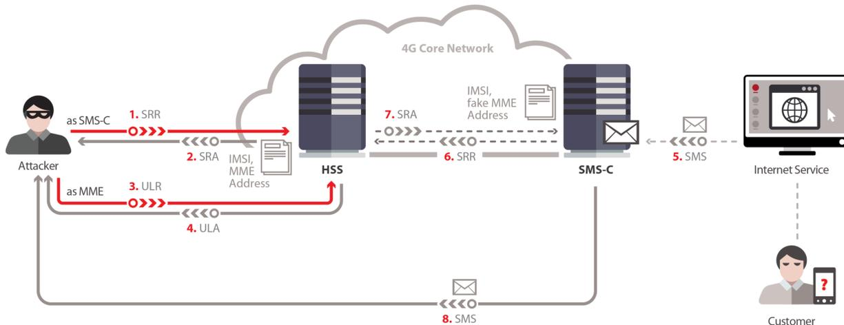
Figure 3 - Example Message flow for intercept of SMS messages
