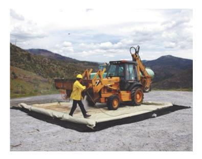
Figure 1. Flexible mat type of vehicle wheel wash, from <a href="http://www.fs.fed.us/eng/pubs/pdf/05511203.pdf">http://www.fs.fed.us/eng/pubs/pdf/05511203.pdf</a>
