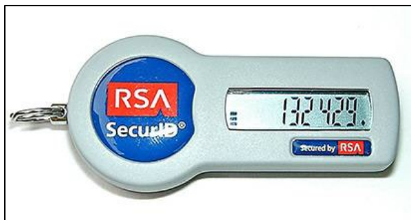
Figure 2: An RSA SecurID® token
