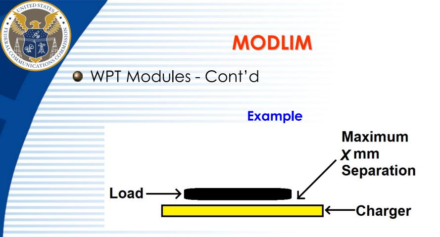
• For this example, let us assume that the charger is incapable of charging at a distance greater than X mm. The sensing circuits do not detect the load and therefore go into low power standby mode.
