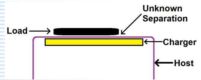
In this condition, the leakage could actually be higher than when originally evaluated stand alone.
