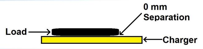
At this separation distance, one would expect the maximum power transfer with the least amount of leakage.
